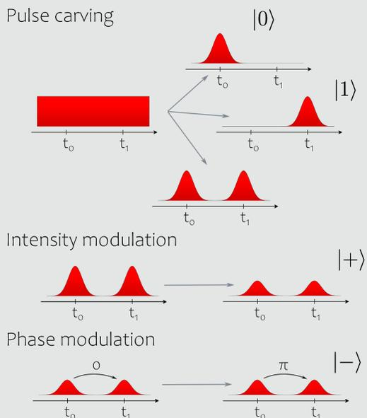
The chip contains three Mach-Zehnder Interferometers (MZIs) and an electro-optic phase modulator (PH MOD) to pulse carve, intensity modulate, phase encode and phase randomise and can be used with various time-bin encoded protocols. All steps contain critical information about the key.
