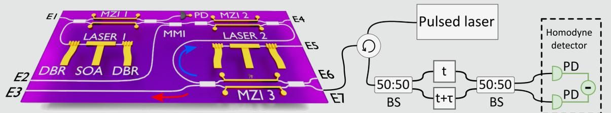
One of the main requirements, is a significant and reliable point of reflection in the system after, from Eve's view, an encoding element. Such a reflection was found and the chip additionally shows a strong reflection where the light is coupled from the chip to the fibre.
