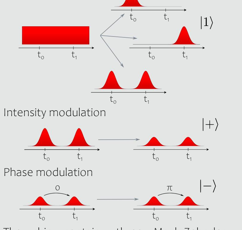
The chip contains three Mach-Zehnder Interferometers (MZIs) and an electro-optic phase modulator (PH MOD) to pulse carve, intensity modulate, phase encode and phase randomise and can be used with various time-bin encoded protocols. All steps contain critical information about the key.
