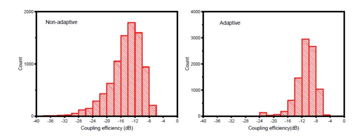
For a normalized atmospheric coherence length of D/r0 = 5.4 (r0 = 7.4 cm @810 nm), the M-SPGD AO system improved the single-mode coupling efficiency from 4.8% to 9.7% and the coupling efficiency fluctuation is obviously suppressed
