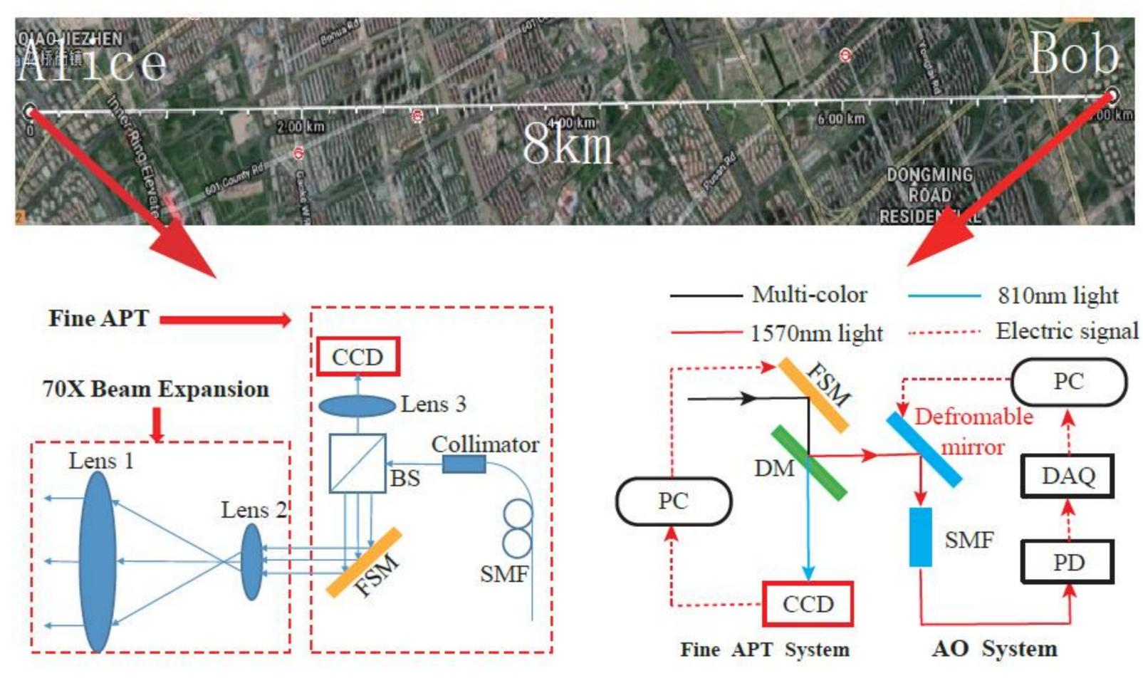
Based on numerous tests over an 8-km free-space link, the results show that our M-SPGD algorithm AO system can effectively improve the SMF coupling efficiency and suppress intensity fluctuations. Moreover, we also used angle-of-arrival fluctuation method to estimate the Fried parameter r0 in order to characterize the strength of the atmospheric turbulence.
