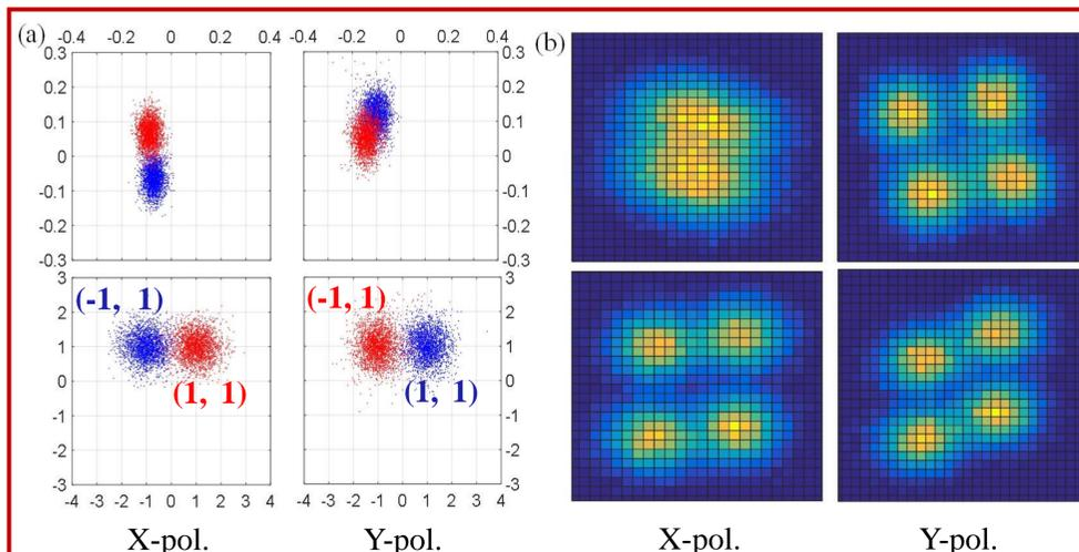
Figure 2 Bob's received (a) reference data and (b) key data without (top) and with (bottom) phase and polarization compensation of X and Y polarization. Blue/red points: the first/second group of reference data.
