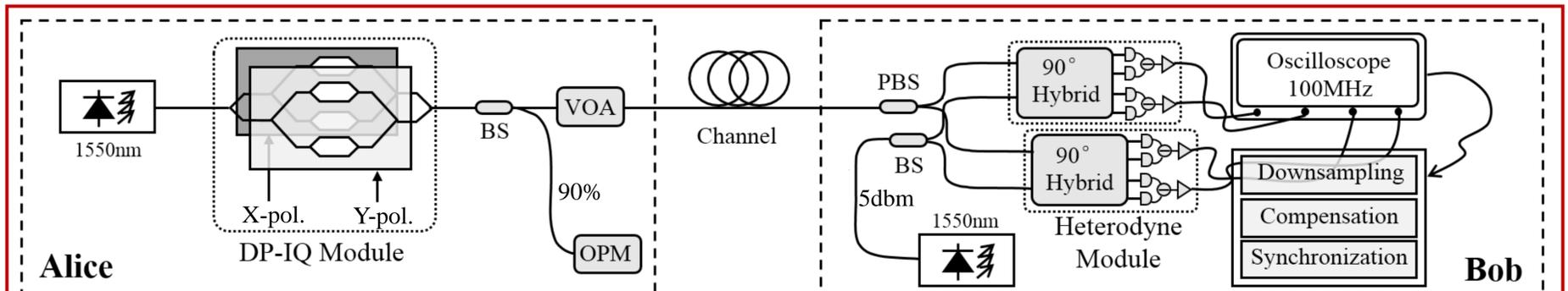
Figure 1 Experimental setup of proposed polarization-multiplexed CV-QKD scheme.
