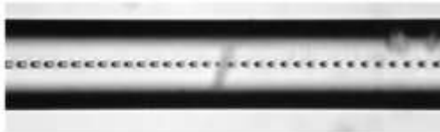
Figure 2 Optical fiber after fuse propagation.
